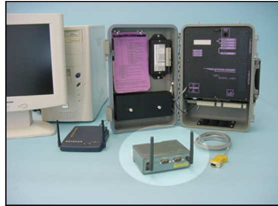
MSS-101-RF, highlighted, shown with Logic Beach HyperLogger, PC and Access Point.
